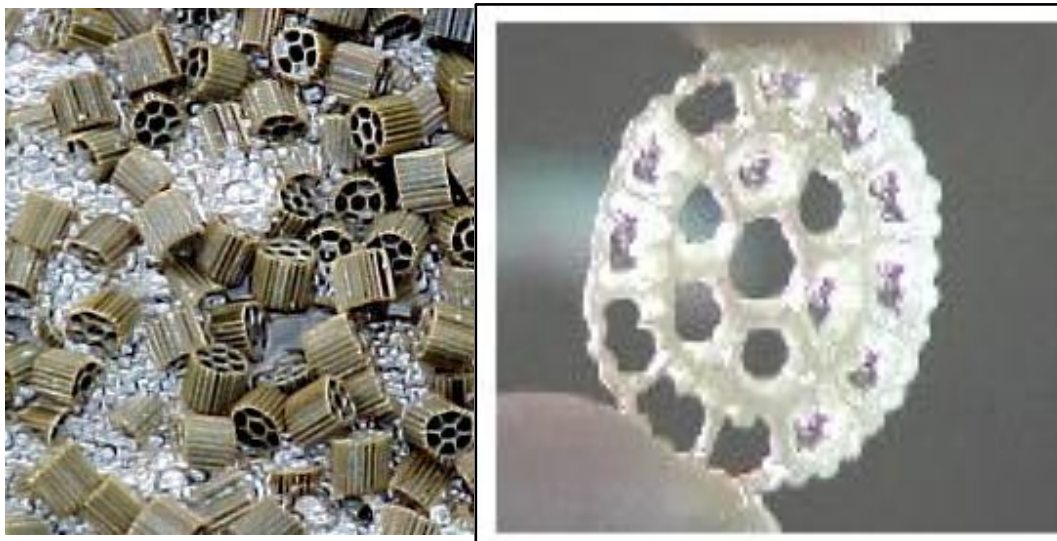
Fig. 8: Media support carriers used in MBBR
