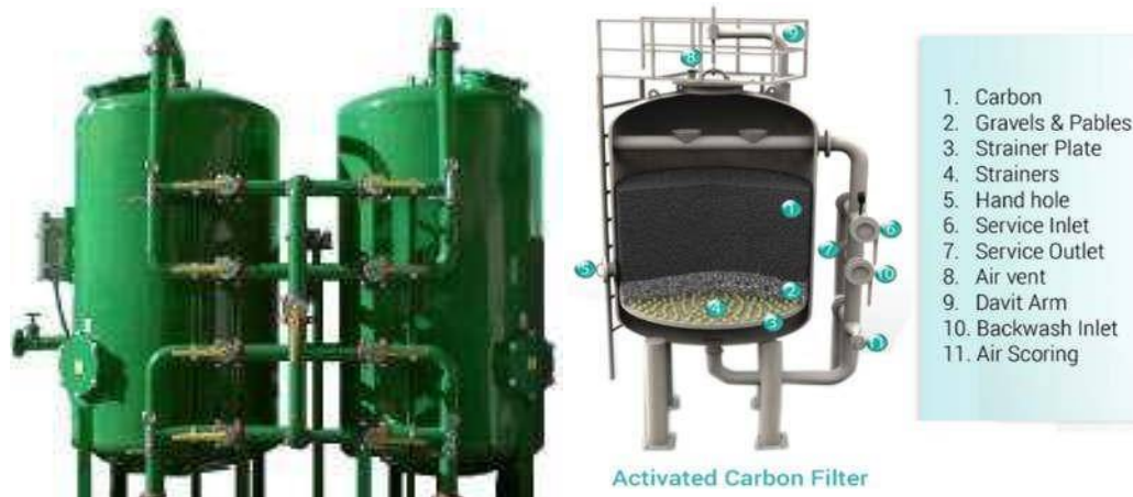
Fig5.4: Activated Carbon Filter
