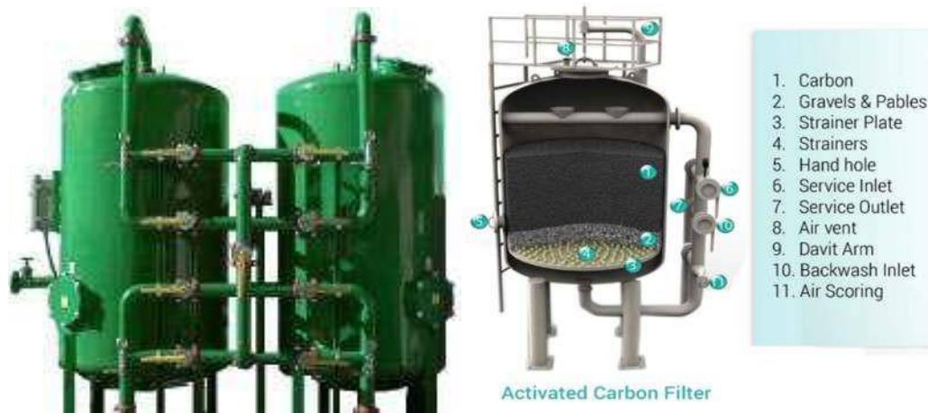
Figure 5.4 Activated Carbon Filter
