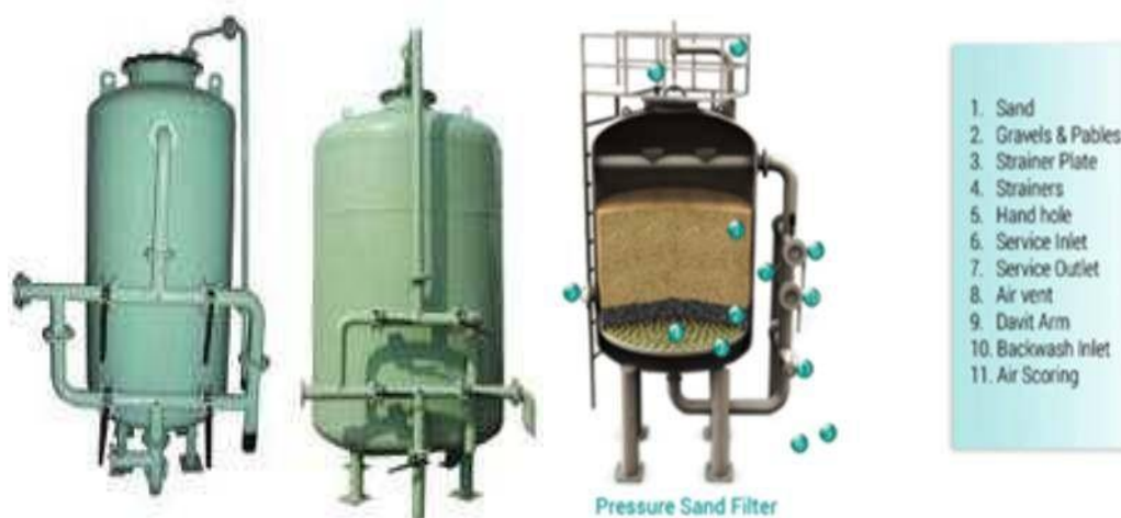
Fig 5.3: Pressure Sand Filter
