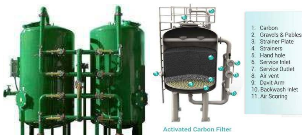
Figure 9 Activated Carbon Filter
