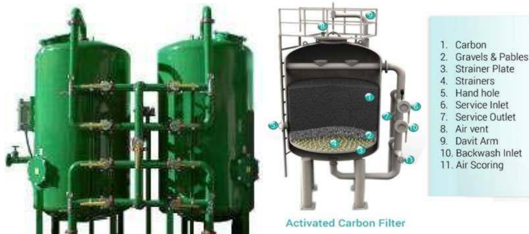
Figure 5.4 Activated Carbon Filter
