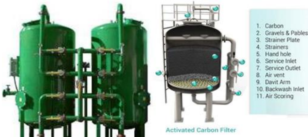
Fig 5.6 Activated Carbon Filter
