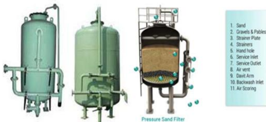
Fig 6.5 Pressure Sand Filter
