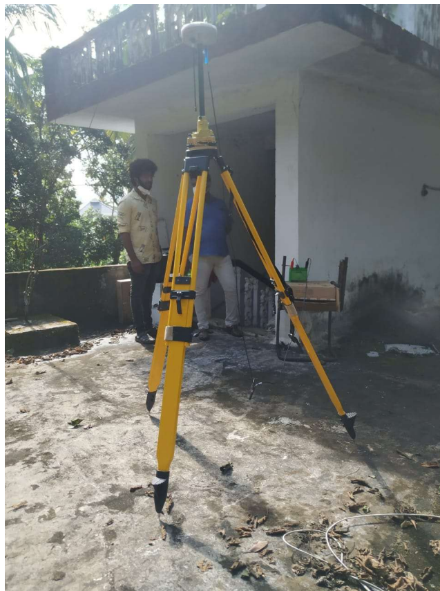
Fig. 10 Base station setting for DGPS survey at Wadakkanchery Municipality
